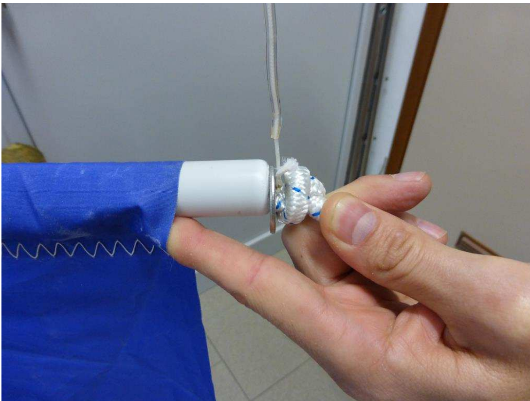
Fig. 12. Attaching the line of the floating foam ball to the “arm” of the drifter.
