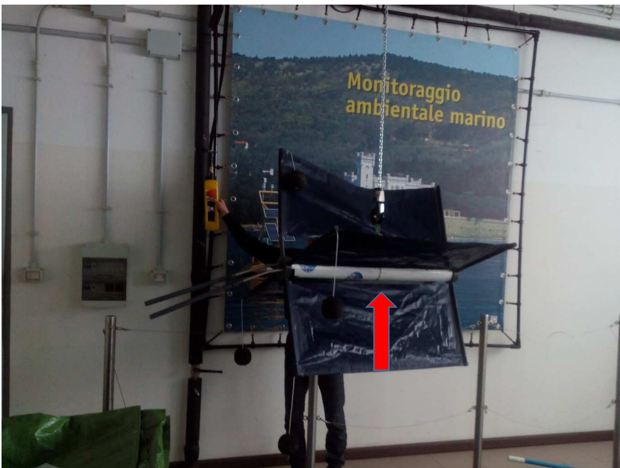
Fig. 20. Center of gravity of the original modified CODE drifter.
