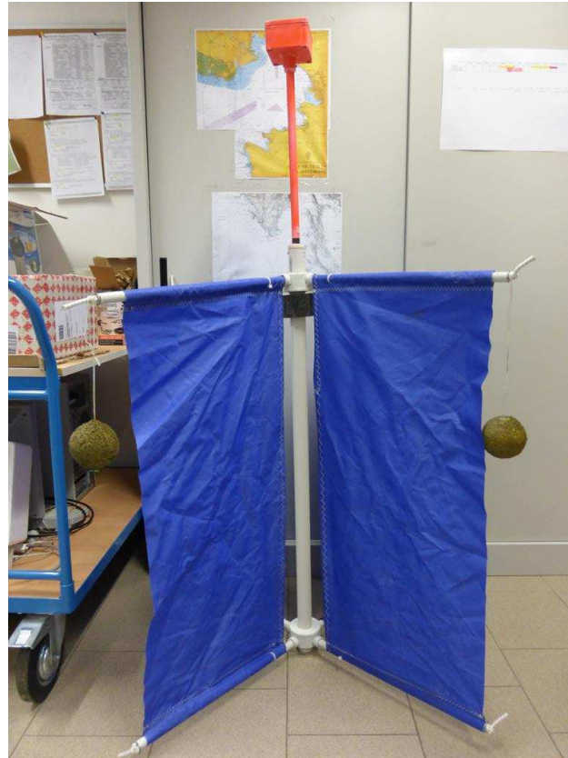
Fig. 13. The drifter fully assembled.
