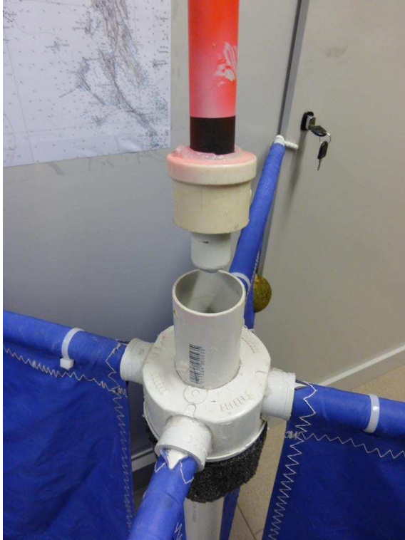
Fig. 9. Conduit reducer fixed on the antenna mast.
