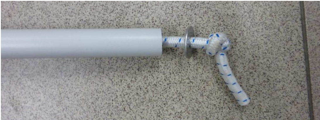
Fig. 7. Knot at one extremity of the elastic cord.
