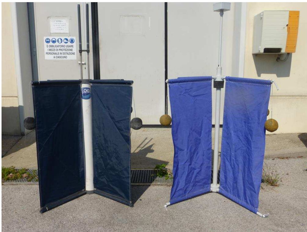
Fig. 14. The OGS low-cost CODE drifter (on the right) and an original modified CODE drifter (on the left).
