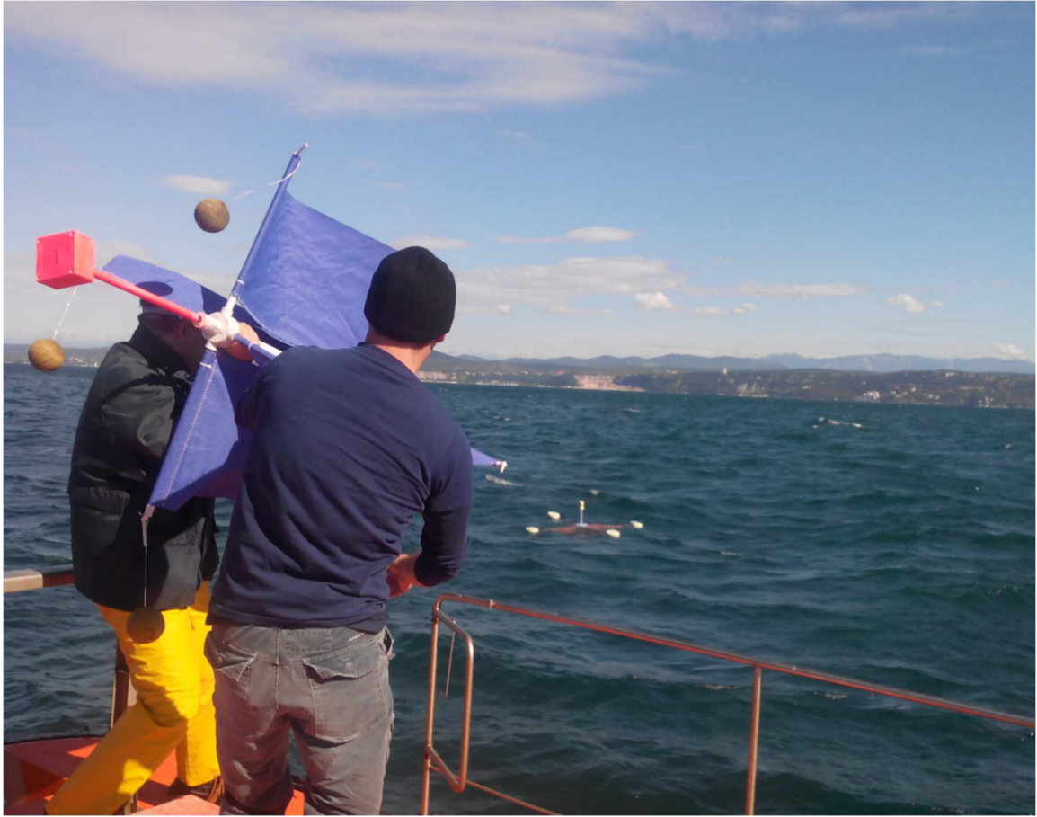
Fig. 17. Deployment of the OGS low-cost CODE drifter.
