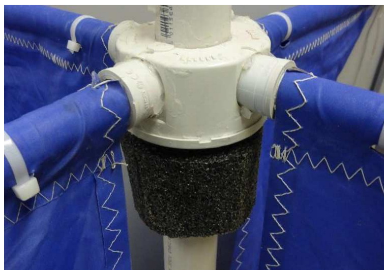
Fig. 6. Foam annulus (in black) providing extra buoyancy to the drifter.
