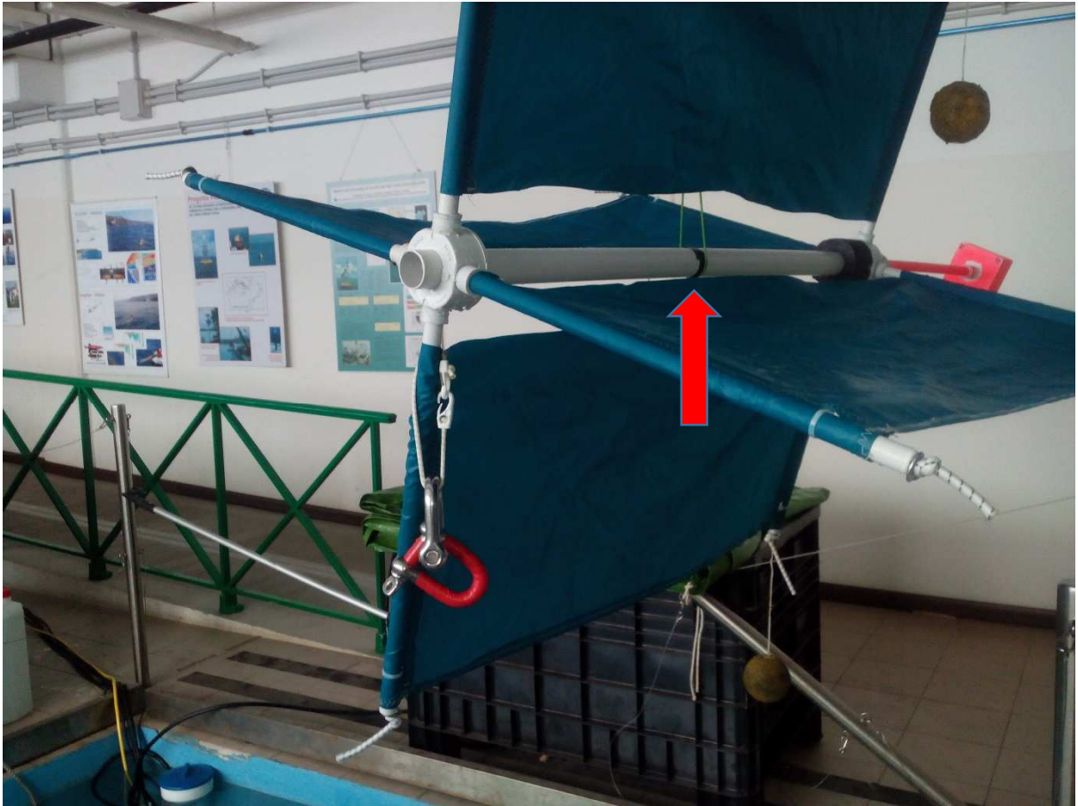
Fig. 22. Center of gravity of the OGS low-cost CODE drifter with the additional weight.
